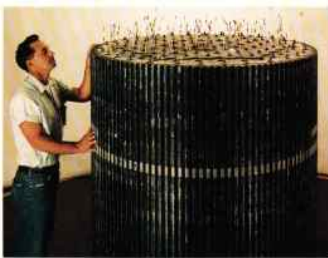
The centerpiece of the Pluto effort, the Tory reactor was designed to be durable but compact enough to fly.
